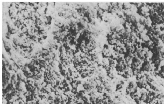
Figure 5 SEM photograph of IPN-2 (magnification 1500x)
