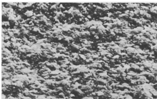
Figure 4 SEM photograph of IPN-15 (magnification 1500x)
